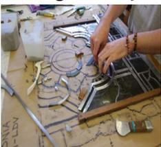
5. Glazing – The trays of glass are then taken from glass conservation to the glazing area and the rubbing is laid onto the table and secured. The pieces of glass are glazed using appropriate sized leads. Once all of the glass has been leaded (glazed) the size of the window is checked against measurements taken of the window openings or to templates made of the irregular tracery or kite openings during removal.
